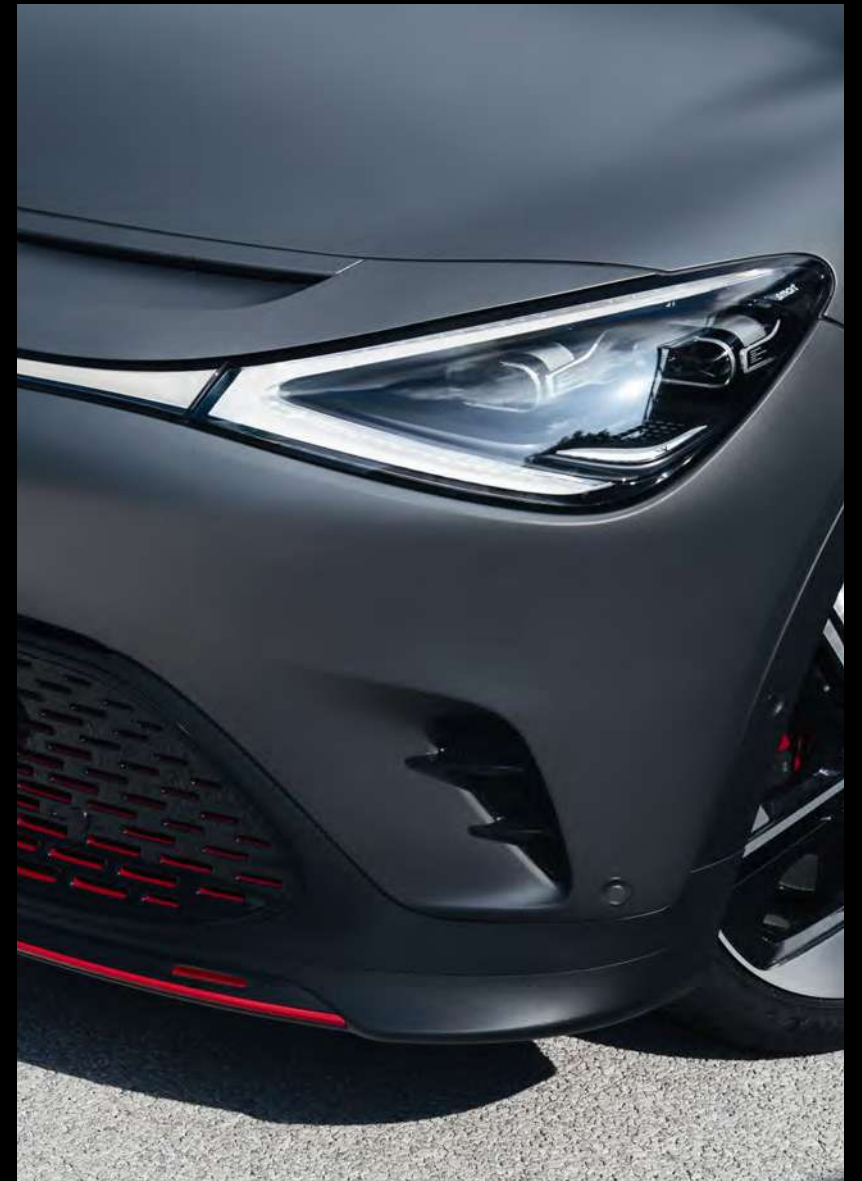
Front Air Diffuser
